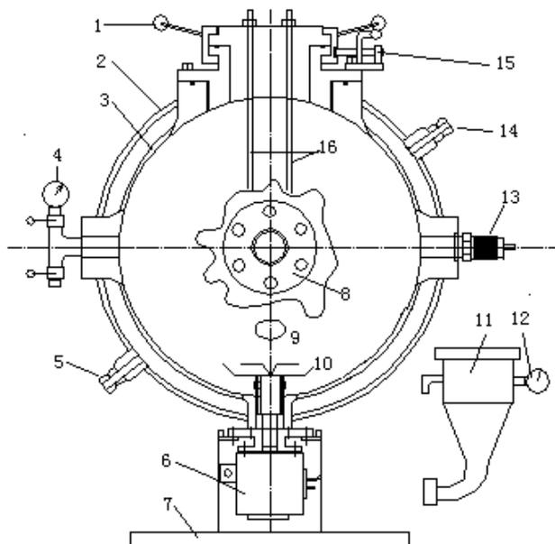
Figure 2 The 20L spherical explosion chamber
