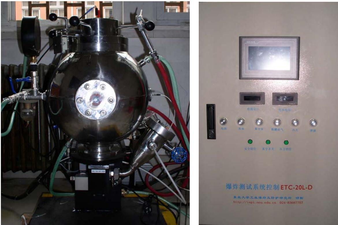
Figure 4 Explosion chamber and control box
