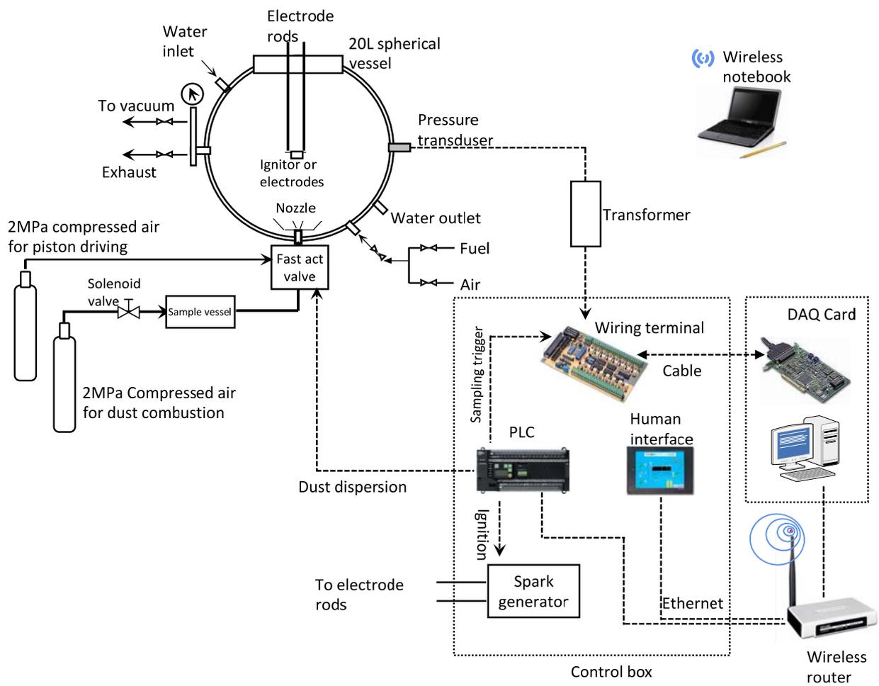
Figure 1 Schematic diagram of 20L explosion test system
