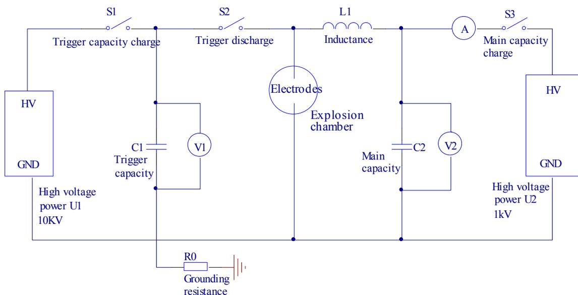
Figure 3 Simplified schematic diagram of electrostatic ignition
