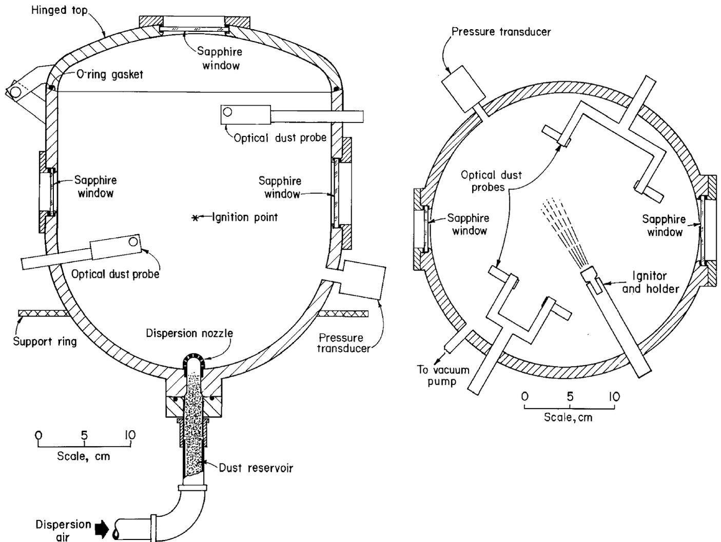
Fig. 1. Vertical and horizontal cross-sections of the 20-L explosibility test chamber.
